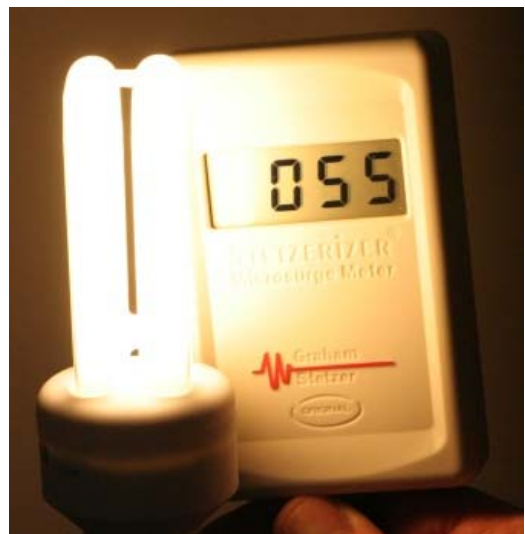
Picture 2: DE monitor and CFL (energy saving light) switched ON
