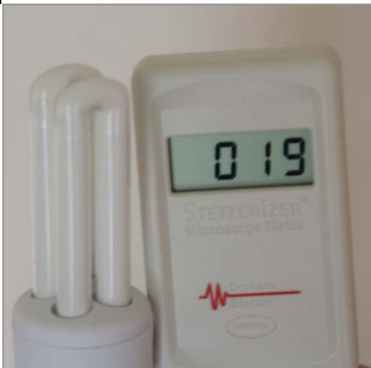
Picture 1: DE monitor and CFL (energy saving light) switched OFF
