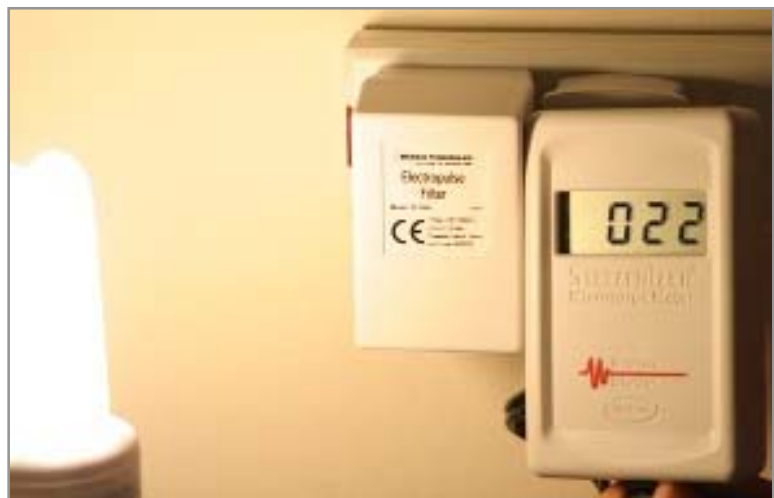
Picture 3: DE monitor and CFL (energy saving light) switched ON plus DE FILTER (reduction from 55 to 22 units.)
